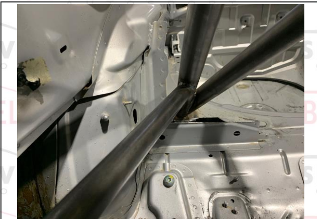
PHOTO 5 REAR BACKSTAY TO BODYSHELL ATTACHMENT
