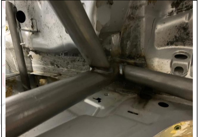
PHOTO 4 MAIN ROLLBAR TO FLOOR ATTACHMENT
