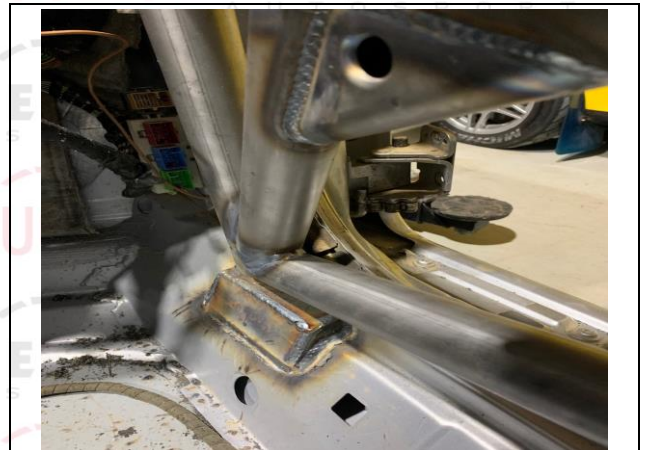
PHOTO 6 FRONT ROLLBAR TO FLOOR ATTACHMENT
